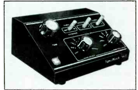
A scanner pre-amplifier can boost incoming signal levels. However, they may also boost the steady noise floor that accompanies weak signals.
