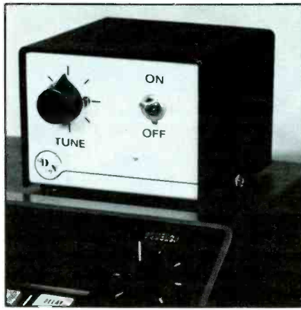
This scanner pre-selector, useful for listeners in downtown areas, allows you to "notch out" interference from adjacent frequencies.
