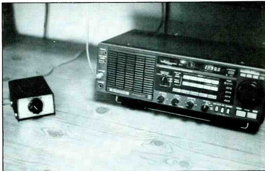
Figure 1. The inexpensive and very useful Flexo switch connected to receiver.
